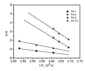
Figure 6. Arrhenius plot for pseudo1<sup>st</sup> order rate constants.
