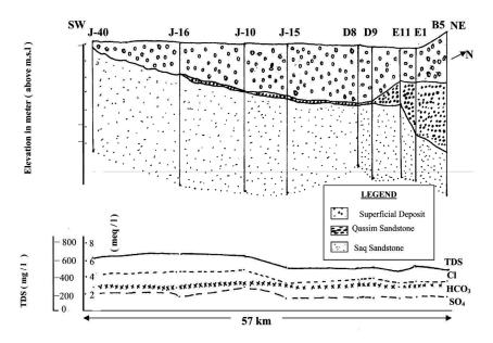
Fig. 4. SW-NE geologic cross-section and a hydrochemical profile along the study area.
