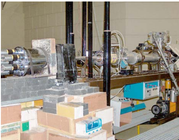
Figure 2: Photograph of the PGNAA setup used to measure prompt gamma ray yield.
