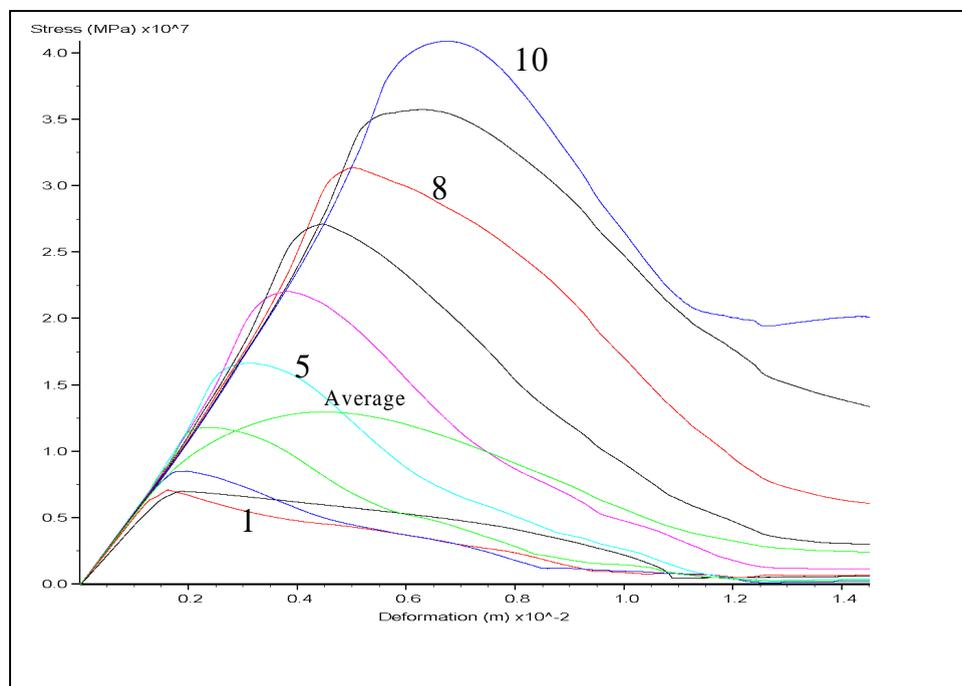
Figure 3: Benchmark element stress versus average pillar deformation (w/h = 2)
