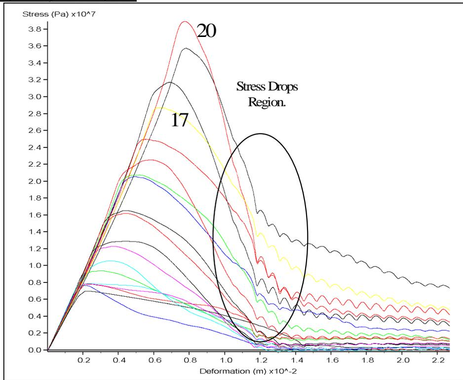
Figure 4: Benchmark element stress versus average pillar deformation ( $w/h = 4$ )
