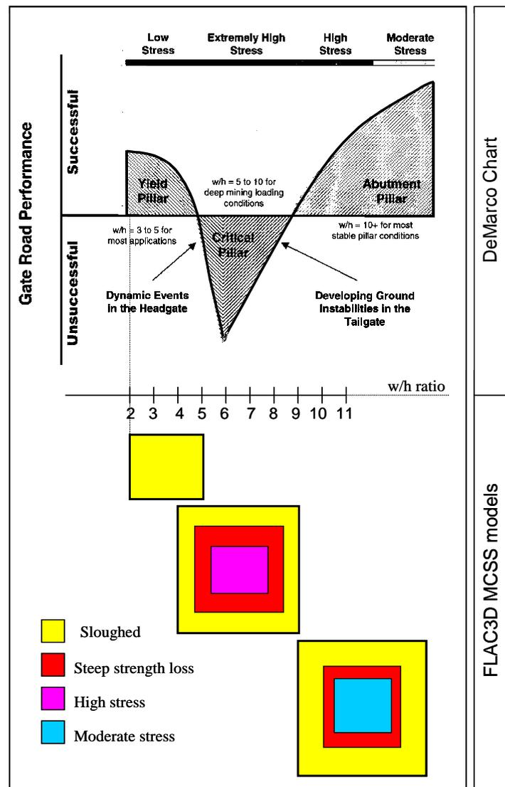
Figure 8: Verification of model results versus DeMarco's conceptual diagram of the instable pillar
