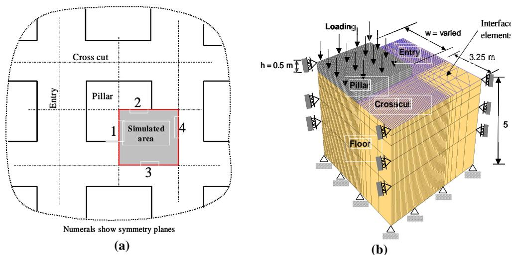
Figure 1: the symmetry lines across a room and pillar mining configuration
