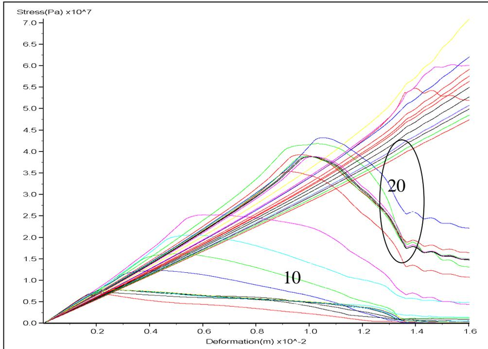
Figure 6: Benchmarked element stress versus average pillar deformation ( $w/h = 9$ )
