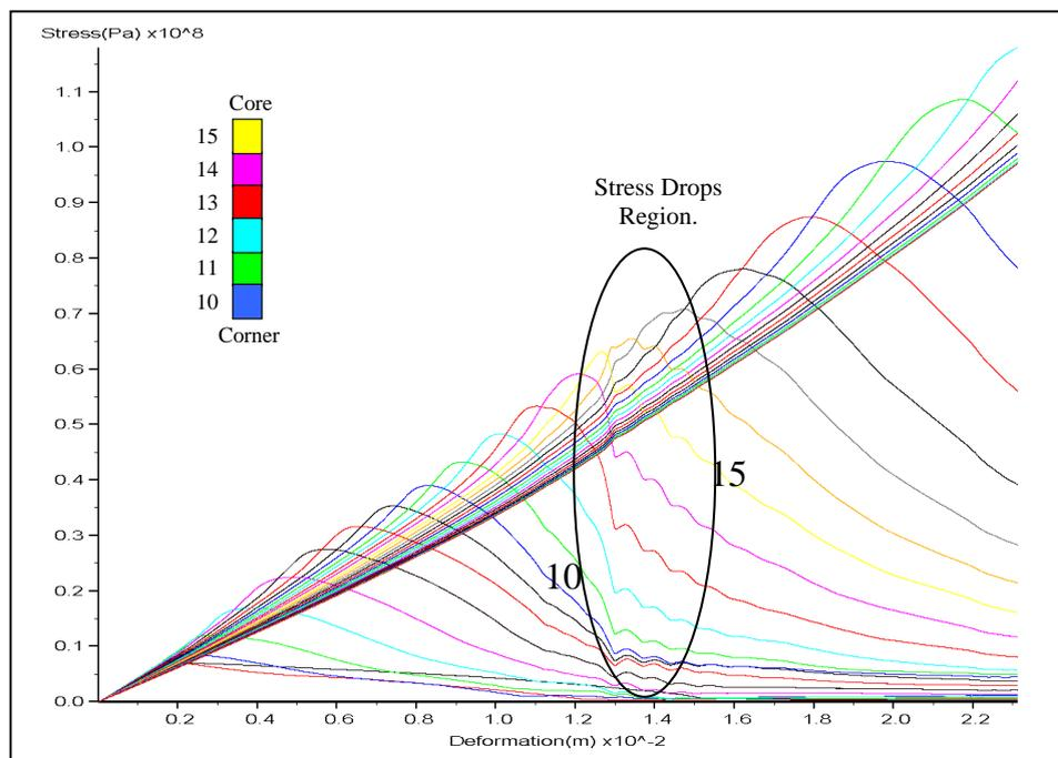
Figure 5: Benchmark element stress versus average pillar deformation ( $w/h = 6$ )
