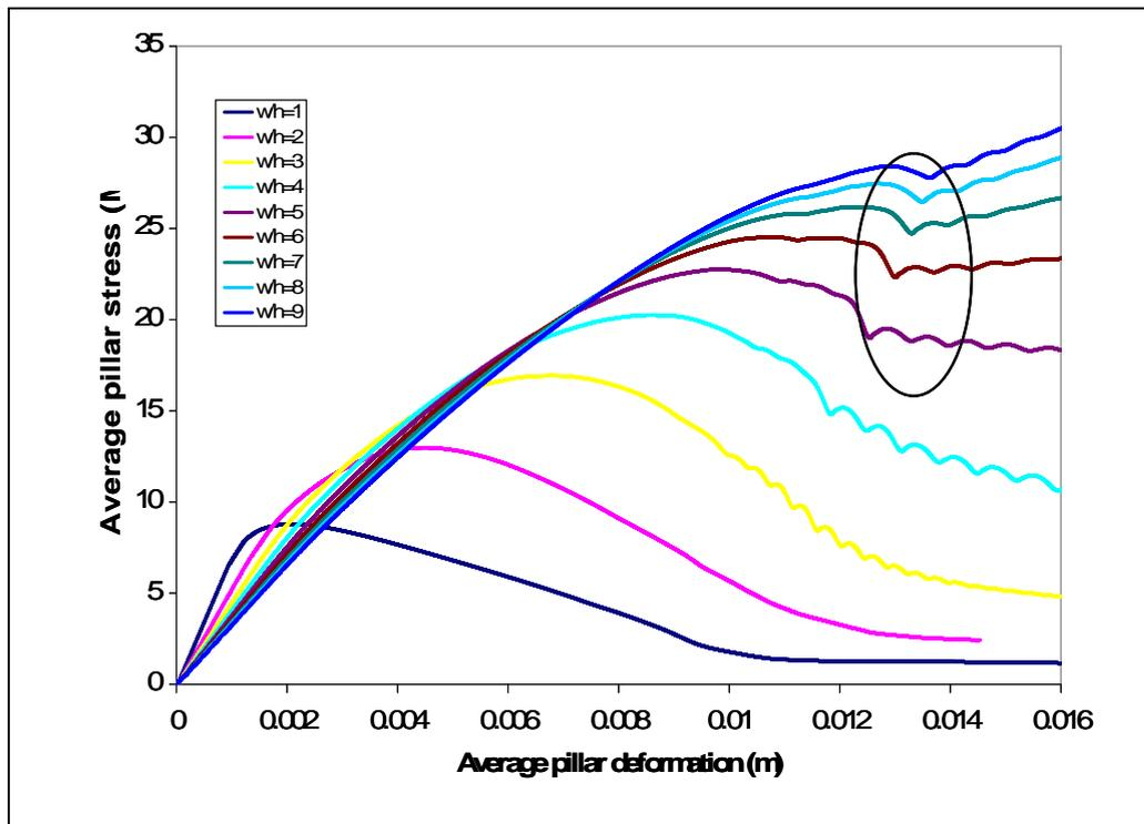
Figure 7: Average pillars vertical stress versus deformation for pillar model
