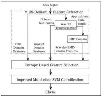
Figure 2 Block diagram of the proposed multi-domain feature extraction, selection and classification of EEG signals
