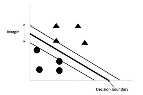
**FIG. 4.** A graphical representation of Support Vector Machines and the linear division of two classes.
