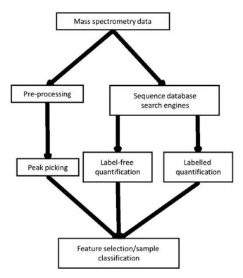
**FIG. 2.** Proteomics mass spectrometry data analysis workflow. The workflow diverges into two sections; the first involves peak picking and application of machine learning directly on mass spectral peaks. This is in comparison to the second section, which involves quantification of proteins, either labeled or label-free, followed by machine learning.
